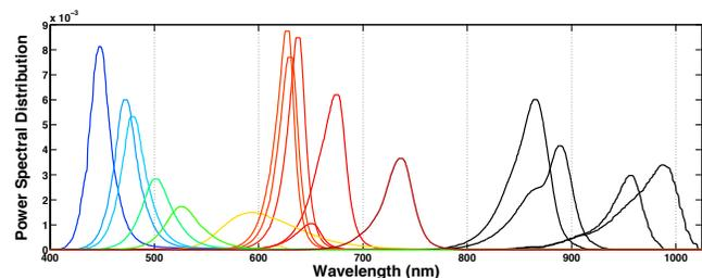
**Figure 3.** Power spectral distribution for the LEDs on HyperCam. The color of the curve corresponds to the color of the wavelength. Black color denotes the infrared wavelengths.
