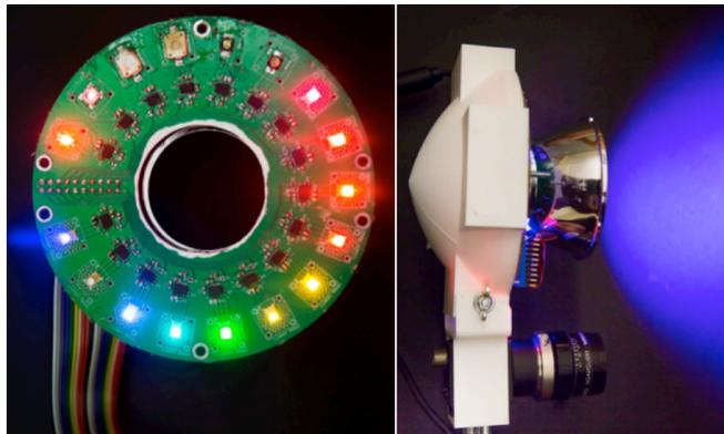
**Figure 4.** (Left) 17 LEDs of different wavelengths form HyperCam’s spectra. (Right) The LEDs shine inside the integrating sphere (white enclosure) and the light comes out of the opening in the center.
