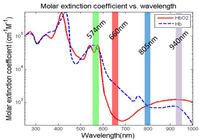
Figure 3. Extinction coefficients for deoxygenated and oxygenated hemoglobin
